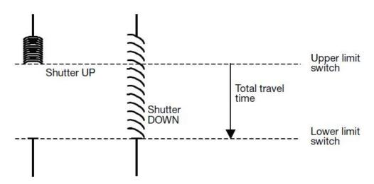
Note: The current position of the Shutter during operation can also be determined with the help of the total move time. It is therefore important to measure and set the total move time as accurately as possible, particularly if the functions "Move to position via a 1 byte value"
