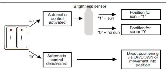
The illuminance sensor senses the intensity of the external light, the button can be switched on, or other control switches on the bus can be used.
