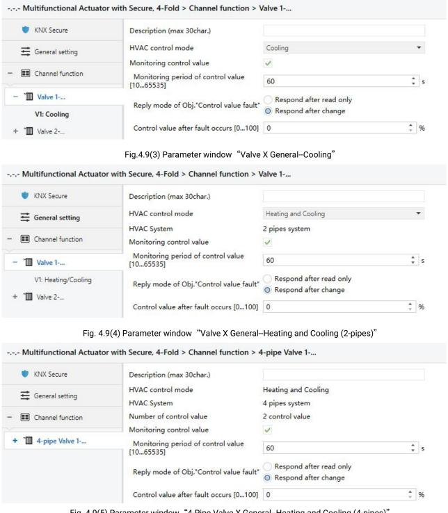
Fig. 4.9(5) Parameter window "4-Pipe Valve X General--Heating and Cooling (4-pipes)"
