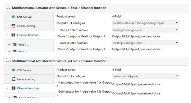
Fig. 4.9(1) Parameter window Channel function--valve type"
