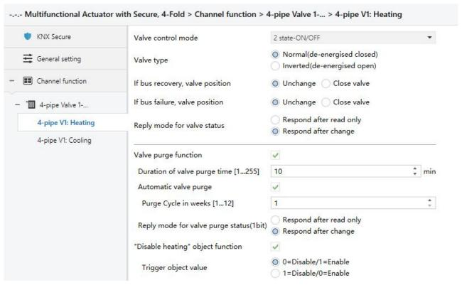
Fig. 4.9.1.1 Parameter window "2 state-ON/OFF"
