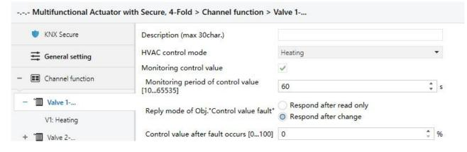
Fig. 4.9(2) Parameter window "Valve X General--Heating"
