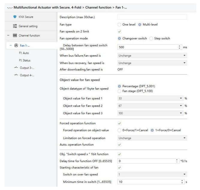
Fig. 4.8.2 Parameter window "Fan type - Multi-level"
