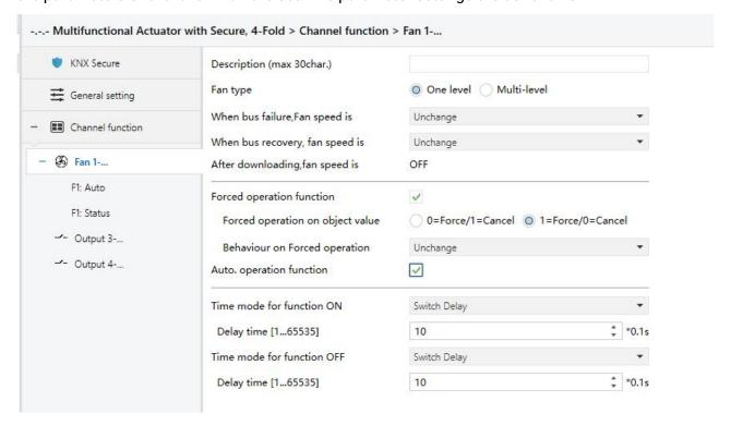
Fig. 4.8.1 Parameter window "Fan type -- One level"
