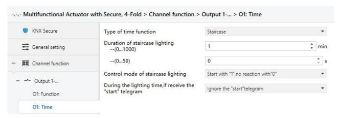
Fig. 4.4.2.3 Parameter window "Ox: Time-Staircase"
