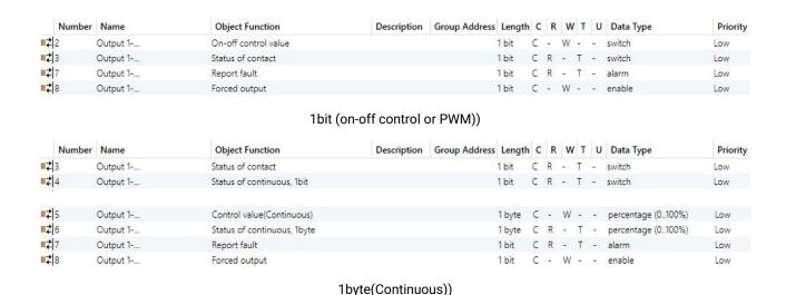
Fig. 5.2.2 Communication object of switch output-heating actuator(without controller)
