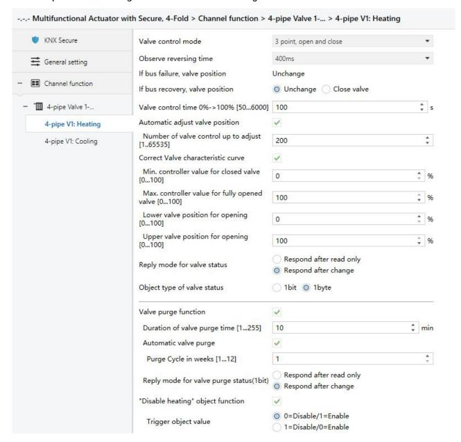
Fig. 4.9.1.3 Parameter window "3 point, open and close"
