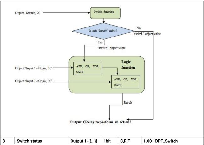
The value of this communication object (Specifically set in the parameter "Object value of switch status" in Figure 4.4 "Output X") Can directly indicate the status of the relay contacts.
