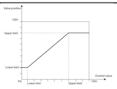
Min. controller value < Max. controller value, if or not, you cannot configure these two parameters in ETS:
