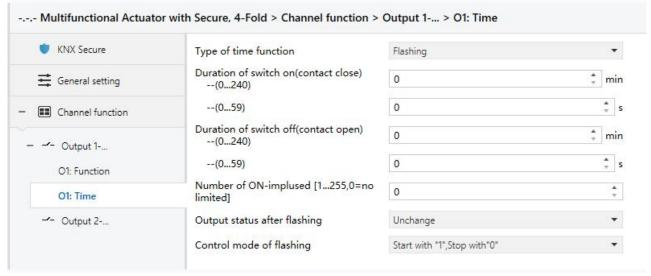
Fig. 4.4.2.2 Parameter window "Ox: Time-Flashing"
