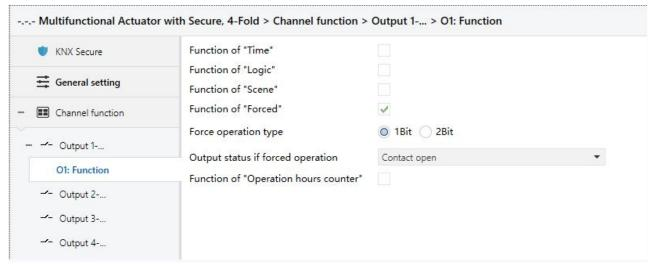
Fig. 4.4.5 Parameter window "Ox: Forced"
