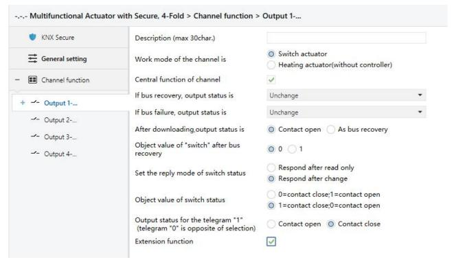
Fig. 4.4.1(1) Parameter window "Output X: Switch actuator"
