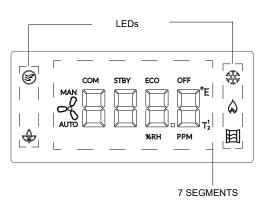
The display has 7 Segments and 5 LEDs described in the below tab:
